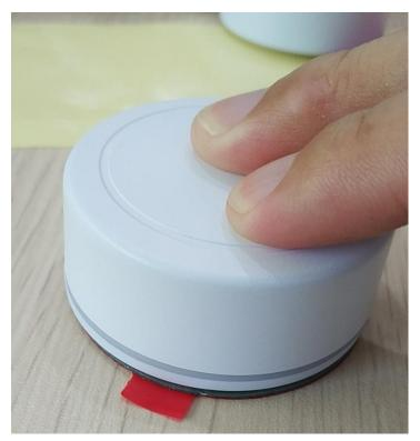
d. Remove the protective oilpaper on the other side of the 3M tape and install VG05 to target installation location (if there is dust or grease stain in the target location, it needs to be cleaned and dried in before install). Press evenly for 5-10 seconds.
