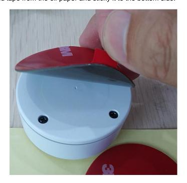
c.Press evenly for 5-10 seconds, make VG05 bottom side and 3M tape fully bonded.
